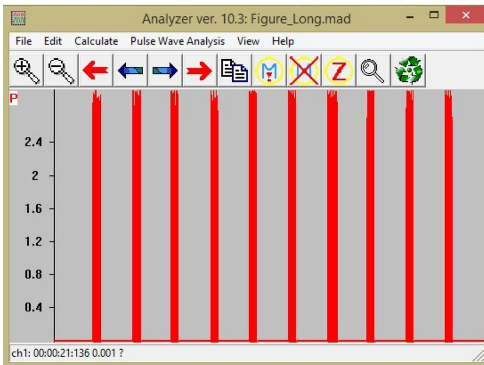
**Fig. 2:** In this example the duty cycle was set to alternating cycles of 5 s on and 25 s off.
