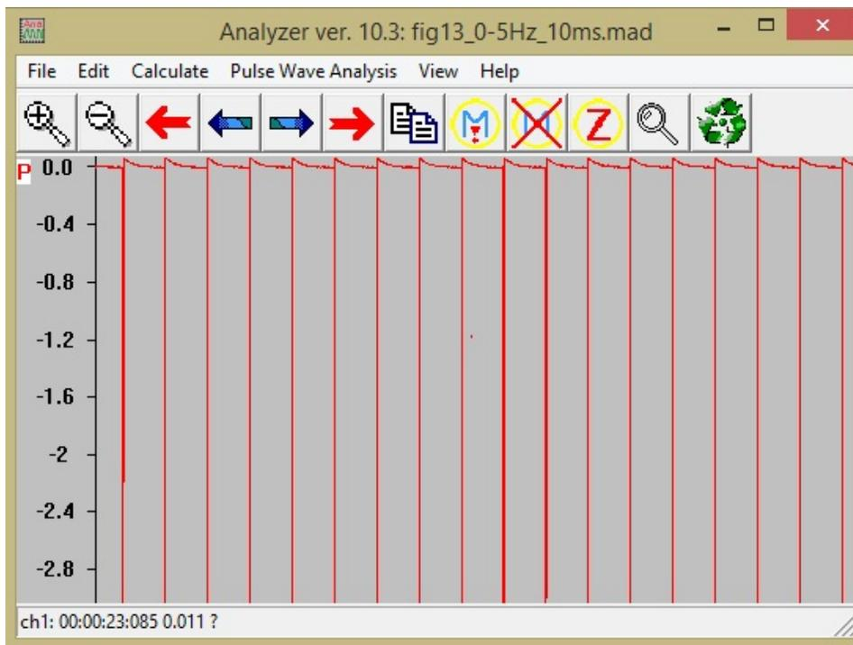
**Fig. 1:** Stimulation at 5Hz, 3V, 1ms pulse width. Note the brief periods of positive voltage following each impulse that effectively charge-balance the stimulation. In this example the voltage at the cathode was recorded relative to the anode. Thus, the impulses show up as negative voltages that depolarize nerve fibers under the cathode.
