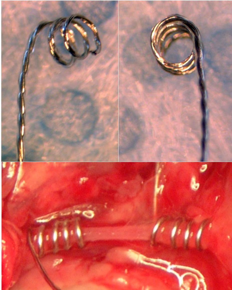
**Fig. 3 top:** Coil electrodes for mouse implants. These coils are made of A-M Systems Catalog #: 793400 electrode wire. This is a PFA-coated, 3-stranded stainless steel wire. The inner coil diameter is 23G (=0.64 mm).
